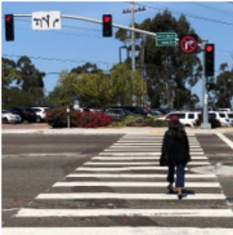
Lead Pedestrian Intervals provide pedestrians a 3-7 second head start when entering an intersection, reinforcing their right-of-way over turning vehicles.
